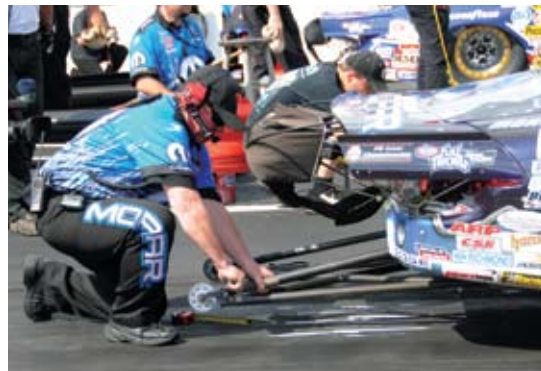
Knowing the differences between rod ends and where they're used is useful information. Rick Jones says, "A two-piece carbon rod end will work fine on a set of wheelie bars for a sportsman-type car, but in a Pro Stock or similarly powered car, it's necessary to use a high quality chromoly end or else they'll break."
