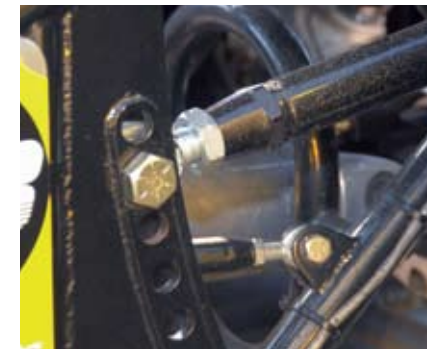
Most rod ends are out in the open, especially in a dragster, meaning they're susceptible to dirt and the elements. Race tracks can be a dusty environment and for this reason, it's important to inspect and clean your rod ends on a regular basis. Should dirt or dust build up between the actual bearing surfaces, it will promote wear.
